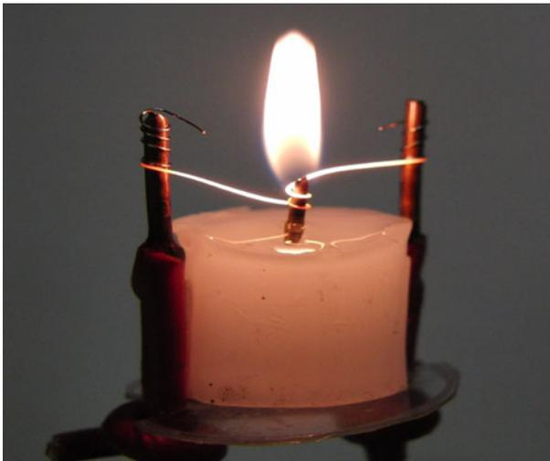
**Fig. 6** A candle with a metallic artificial wick heated using an electric current
