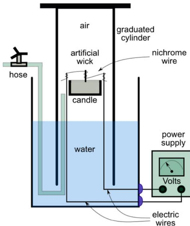
**Fig. 3** Experimental setup used in our closed volume artificial wick candle experiments
